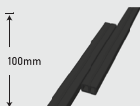
Minimum overlay when connecting supports
